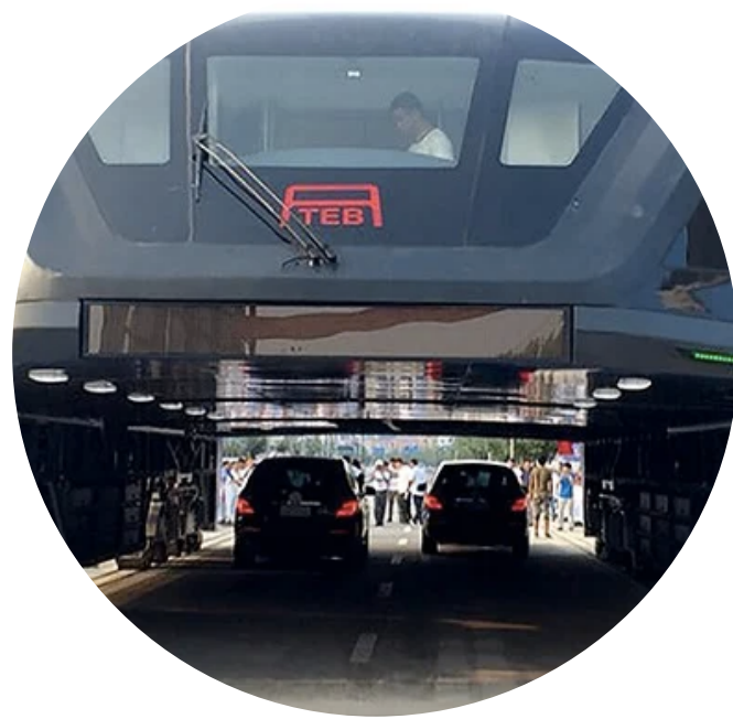
Transit Elevated Bus
